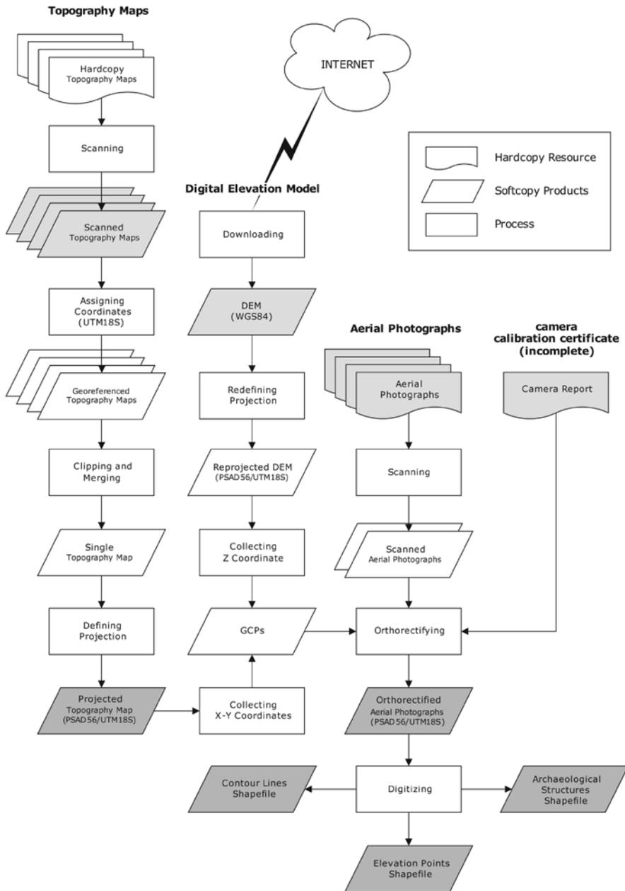
Figure 14.1. The workflow of prototype map creation (Phase I).
