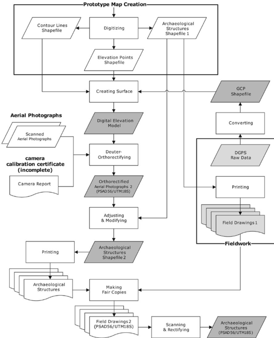
**Figure 14.2.** The workflow of post-fieldwork data processing (Phase III).
